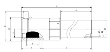
PE 100 SDR 11 Maximum working pressure 10 bar (gas)
