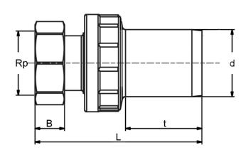
PE 100 SDR 11 Maximum working pressure 16 bar (water)
