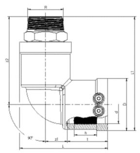
PE 100 SDR 11 Maximum working pressure 16 bar (water)
