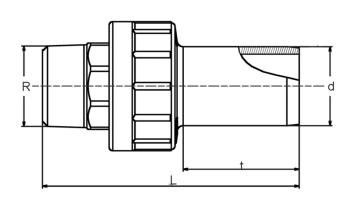
PE 100 SDR 11 Maximum working pressure 16 bar (water)/5 bar (gas)
