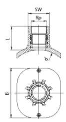
PE 100 SDR 11 Maximum working pressure 16 bar (water)/10 bar (gas)
