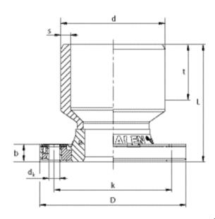
PE 100 SDR 11 Maximum working pressure 16 bar (water)
