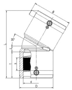
PE 100 SDR 11 Maximum working pressure 16 bar (water)/10 bar (gas)
