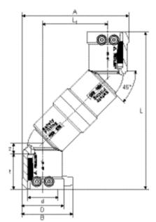
PE 100 SDR 11 Maximum working pressure 16 bar (water)/10 bar (gas)
