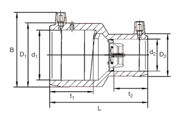
PE 100 SDR 11 Maximum working pressure Type Z: 5 bar (gas), Type D: 1 bar (gas)
