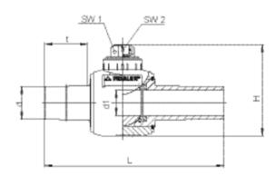
PE 100 SDR 11 Maximum working pressure 10 bar (gas)
