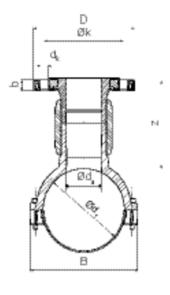
PE 100 SDR 11 Maximum working pressure 16 bar (water)
