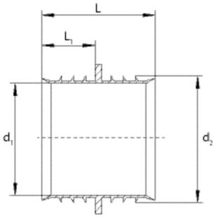
Only suitable for pipes SDR 11
