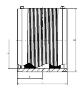
PE 100 SDR 17  $$\operatorname{Maximum}$  permissible working pressure 10 bar (water / sewage)
