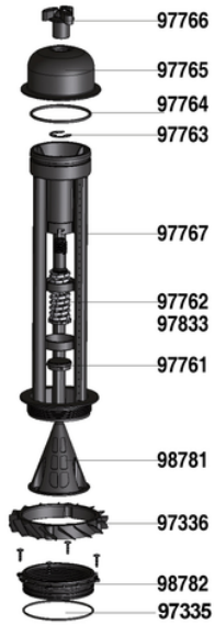
Deflector for hydroCICLONic filter
