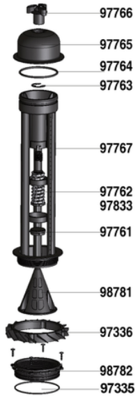
Axis/spring wih hydraulic piston
