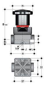
**CMIV** Compact diaphragm valve with female ends for solvent welding, metric series
